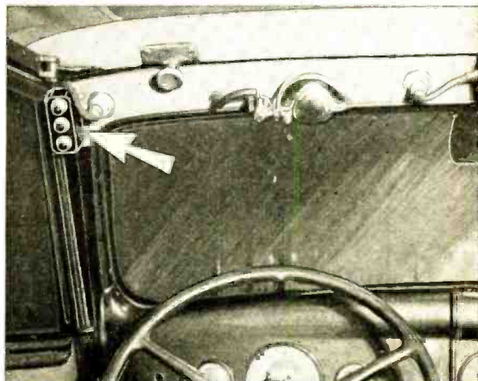
After experimenting with several different positions in the car it was found that greatest visibility and convenience to the driver were obtained when the Stop, Caution and Go signals were attached to the left windshield post of the car. Leads connect the signals to control equipment under this instrument panel.
