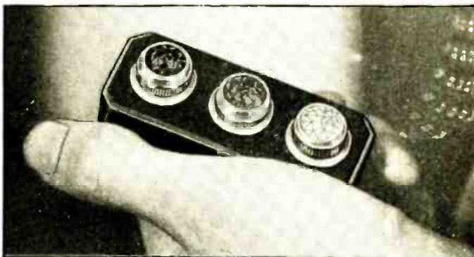
These are the red, amber and green signals which mount on the left windshield post at the eye level of the driver. Selective devices attached to the receiver pick off the audio frequency control tones which individually actuate these Stop, Caution and Go signals.
