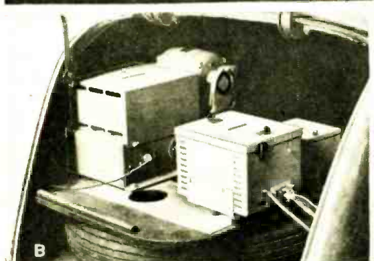
Upper-Left: New 25-watt police radio xmtr, as set up on a Despatcher's desk in headquarters. Lower Left: The 15-watt crystal-control UHF receiver & dynamotor, mounted in the rear trunk of a 1938 Ford. The receiver is in the foreground. Above: Control unit & handset mounted on dash of same car. All equip't in this layout is G-E except handset, which is by Automatic Electric Co.
