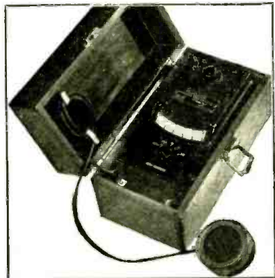
Photoelectric light meter. (1700)
